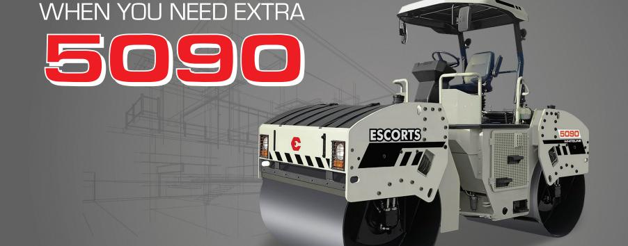
Escorts Engine: 75 HP | Static Linear Load 27.7 kg/cm | Total Applied Load 22.4 Ton
